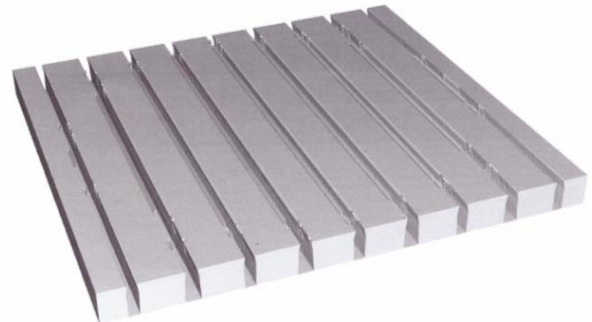
Fig. 15. 3D resist profiles of the exposed microstructures (parallel lines) at exposure with ion beams of parameters as in the Fig.14. The external proximity effect is not observed.
