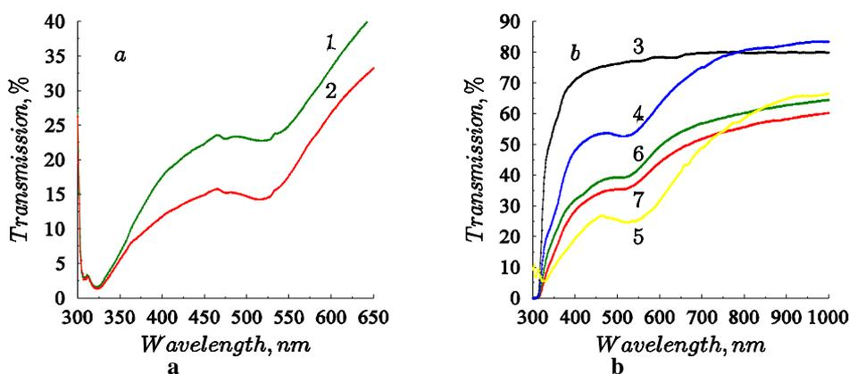
Fig. 1. Optical transmission spectra : (a) - for 10 wt % SiO<sub>2</sub> - 0,3 wt% AuNPs-AmAc nanocomposite (1- monomer, 2-polymer); (b) - for SiO<sub>2</sub>-0,2 wt% AuNPs-UDMA nanocomposites: (3) - 10 wt% SiO<sub>2</sub>/UDMA polymer; (4) 26wt% SiO<sub>2</sub>/ 0.2 wt% AuNPs/ UDMA, monomer; (5) - 26wt% SiO<sub>2</sub>/ 0.2wt% AuNPs/ UDMA, polymer; (6) - 10wt% SiO<sub>2</sub>/ 0.2wt% AuNPs/ UDMA, monomer; (7) - 10wt% SiO<sub>2</sub>/ 0.2wt% AuNP/ UDMA, polymer
