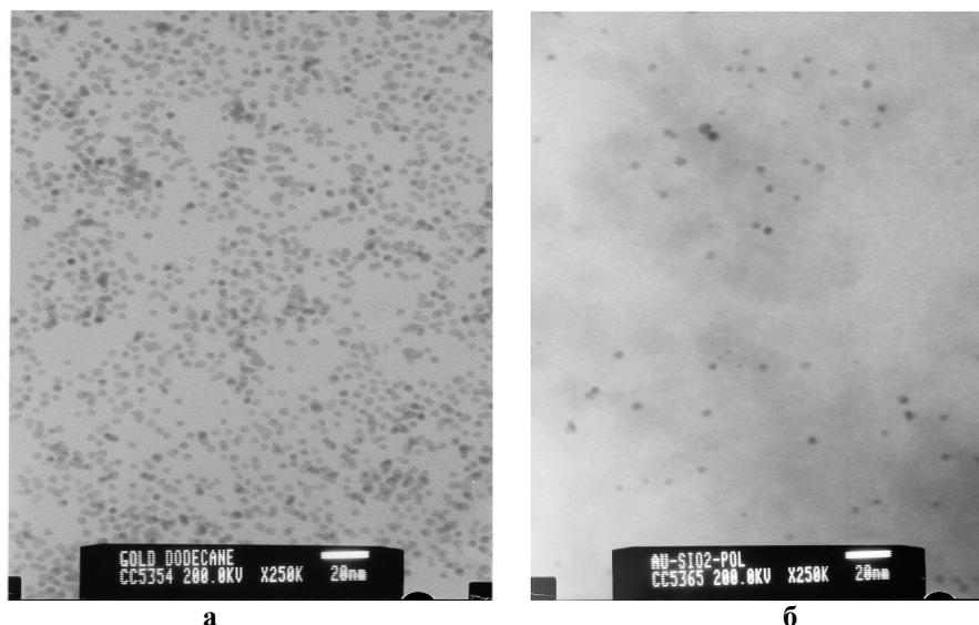
**Fig. 2.** TEM pictures of AuNPs in different matrix: Material – **a)** UDMA/ 0,2 wt% AuNPs/ 10% SiO<sub>2</sub> NPs; **b)** 0,2 wt% Au NP/UDMA with SiO<sub>2</sub>
