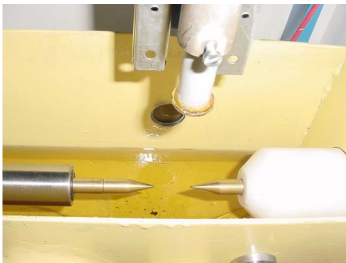
Fig. 2. Schematic of a point-point grounded spark gap 1 – structure fastening the gap, 2 – point and point electrodes
